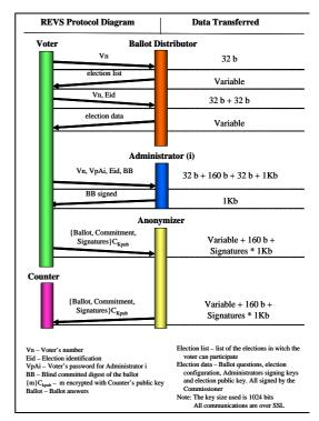
Figure 3 - REVS protocol details
