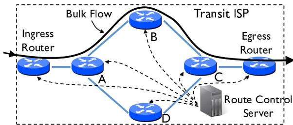
**Figure 1: Deployment of NetEx in a transit ISP:** Bulk transfers are routed through the ISP along the routes computed by the Route Control Server (RCS).
