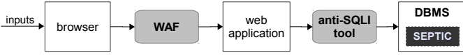
Fig. 7: Placement of the protections considered in the experimental evaluation: SEPTIC, anti-SQLI tools, and WAF.
