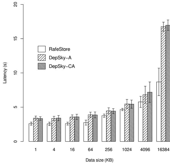
Figure 3: Latencies and data sizes, Configuration 1.
