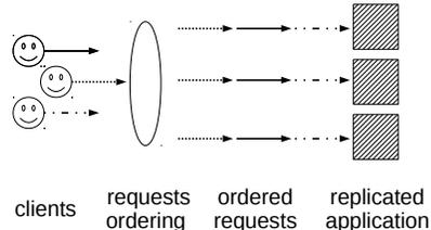
Fig. 3: Ordering requests for simultaneous clients accessing a replicated stateful application.
