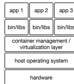
Fig. 1: Container-based Virtualization.
