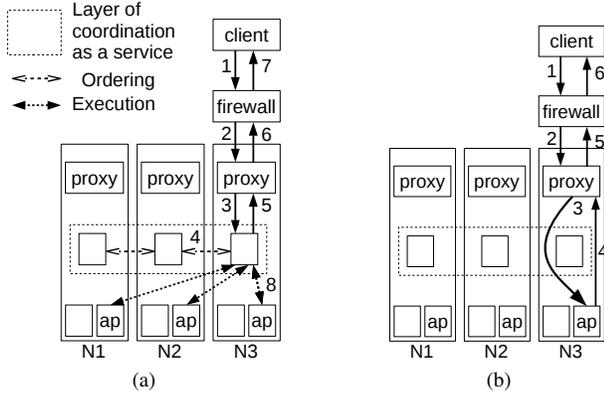
Fig. 4: Koordinator: (a) coordinating updates and (b) direct reading in the replicated application.
