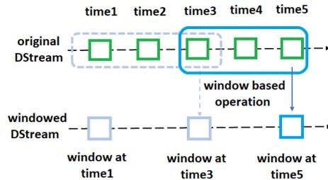
Fig. 6. Spark streaming window operations (adapted from [1])
