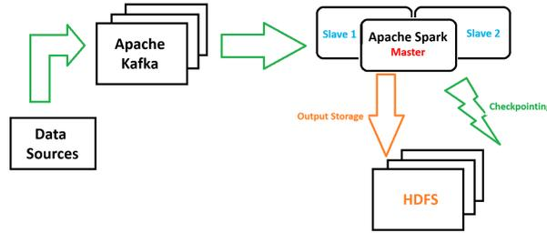
**Fig. 3.** System architecture
