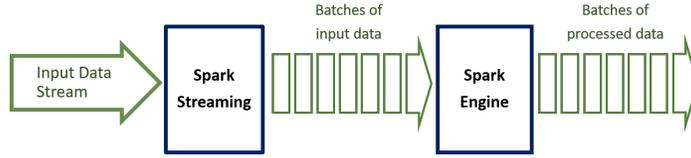
Fig. 5. Spark streaming process
