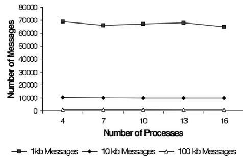
**Figure 1. Number of contexts in the *context buffer* when a buffer overflow happens and the system blocks (Byzantine faultload)**
