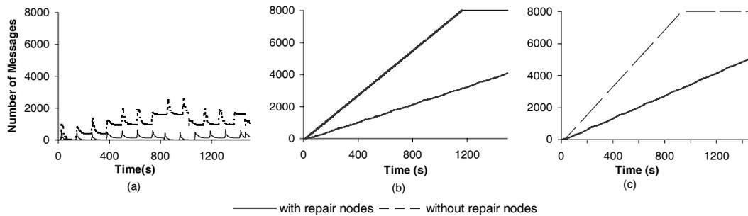
**Figure 4. Buffer occupation measured with (a) fault-free, (b) fail-stop and (c) Byzantine faultload**
