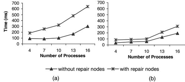
**Figure 2. Time to discard the first data message, measured with (a) fail-stop and (b) Byzantine faultloads, with and without repair nodes**
