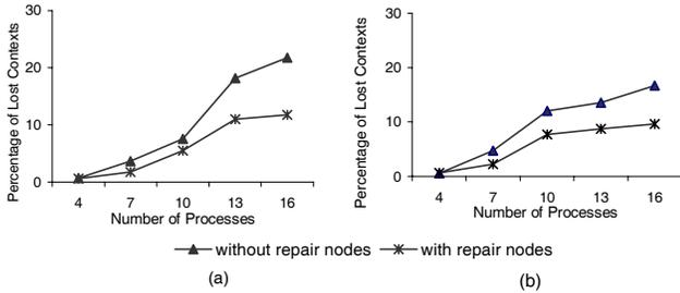
**Figure 3. Percentage of data messages lost measured with (a) fail-stop and (b) Byzantine faultload, with and without repair nodes**
