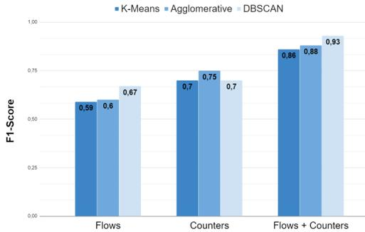
Fig. 3. Comparison of F1-Scores when using only flow-based features, performance counters-based features, and the combination of both (hybrid dataset).
