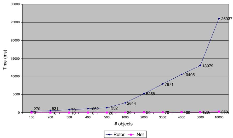
Figure 8: Test-graph serialization times in Rotor and in .Net commercial version.
