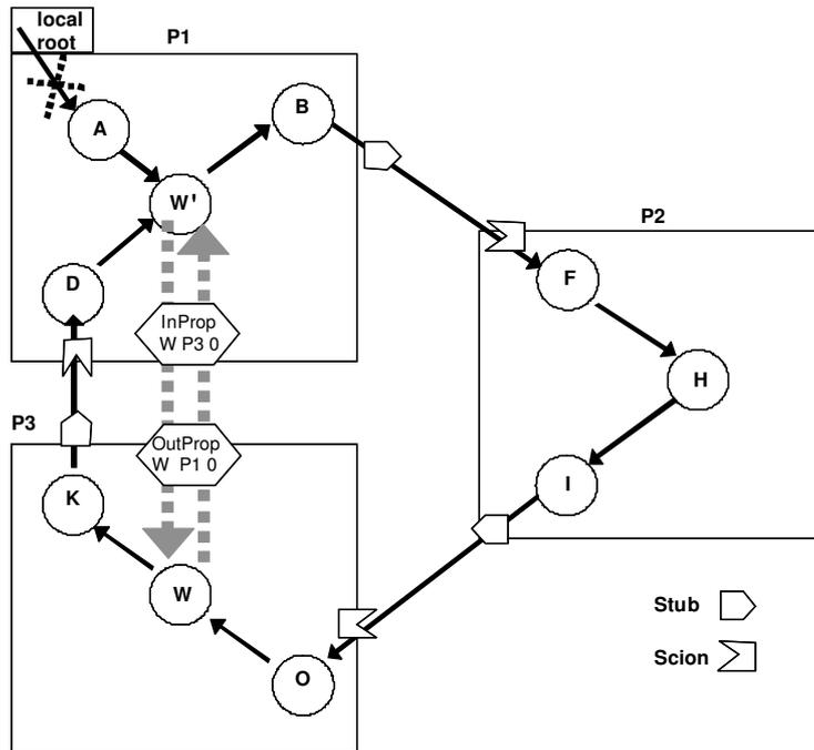
Figure 2: Cyclic distributed garbage comprising replicated objects. Object  $W$  has been previously replicated from process  $P3$  to process  $P1$ .
