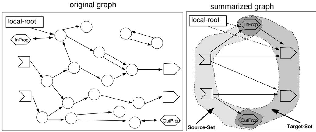
Figure 3: Summarization of an object graph into *Source-Set* and *Target-Set*.
