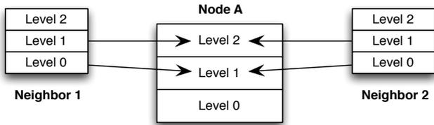
**Figure 1: Example of a node A creating a single Attenuated Bloom Filter by merging each Level  $i$  of its neighbors' Attenuated Bloom Filters into Level  $i + 1$ .**
