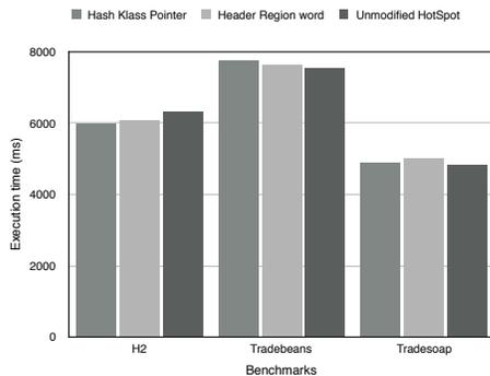
Fig. 12. Execution times over three benchmarks — H2, Tradebeans and Tradesoap — in respect to the BDA-heap
