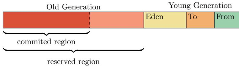
Fig. 1. Parallel Scavenge heap layout
