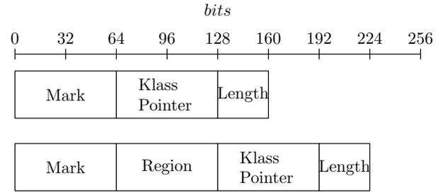
Fig. 6. Layout of an array object header with an added word for region-space indexing
