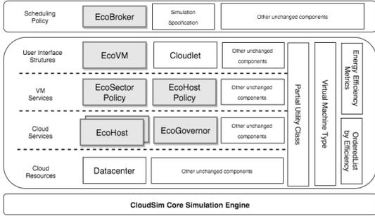
Figure 5: Highlighted extensions to the CloudSim simulation environment
