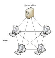
Figure 2.8: Peer-to-Peer with Central Arbitrer Architecture
