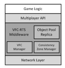
Figure 3.9: Server node Layered Architecture
