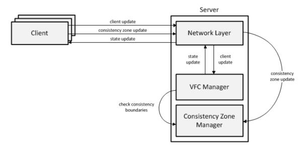
Figure 3.12: Client-Server Message Flow
