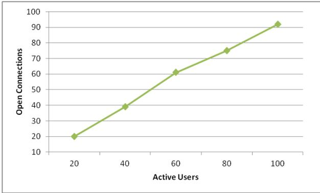
**Figure 12: Open connections growth with the number of active users**
