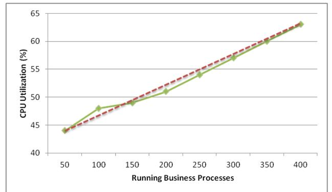
Figure 7: CPU utilization growth with the number of running business processes
