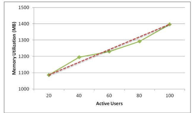
**Figure 10: Memory utilization growth with the number of active users**
