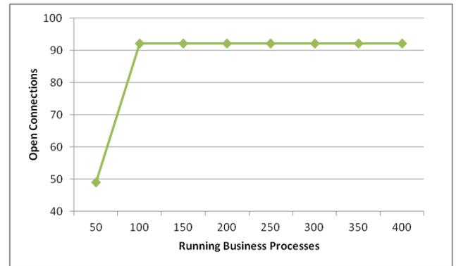
**Figure 11: Open connections growth with the number of running business processes**
