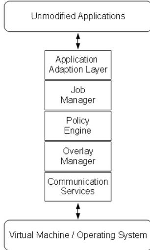
Fig. 2. System Architecture
