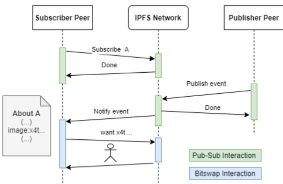
Figure 1: Peers interacting with the current static IPFS layer and a dynamic pub-sub layer
