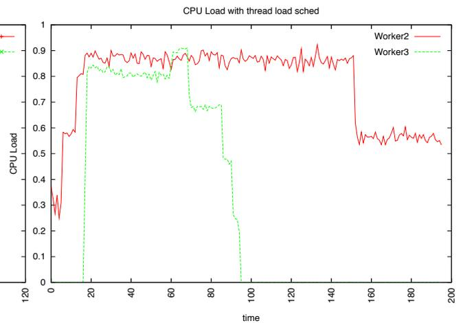
Figure 5.12: CPU Load over time for scheduling based on thread load
