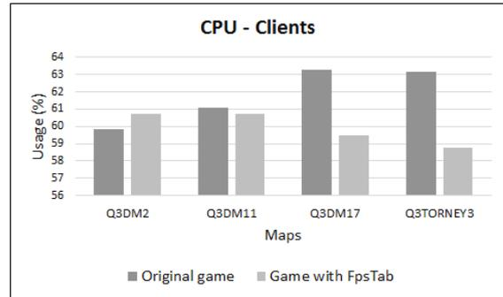
Figure 14: CPU usage by clients. Comparison by map type.
