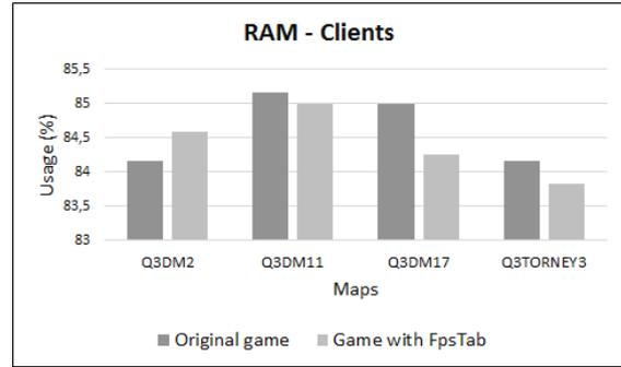
Figure 15: RAM usage by clients. Comparison by map type.
