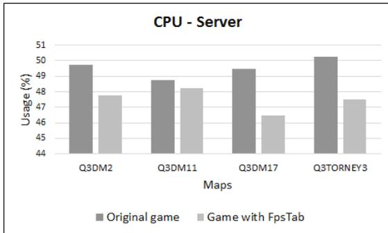
Figure 13: CPU usage by server. Comparison by map type.
