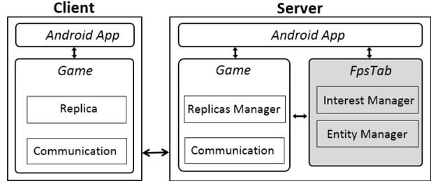
Figure 5: Overall system architecture.
