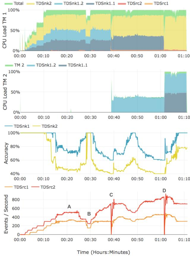
**Figure 3: Execution of the TD application where all sinks have the same priority. First two charts show the CPU load of each TM and their executing tasks. Third and fourth charts show the application sinks' accuracy and the application throughput for each input Kafka topic, respectively.**
