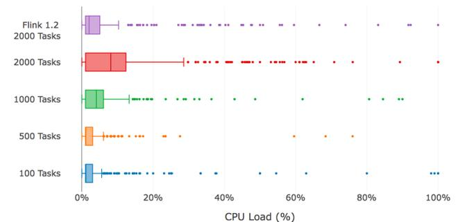
**Figure 6: CPU Load of the JM for different amounts of executing tasks, with two TMs, and comparison with Flink 1.2 release.**
