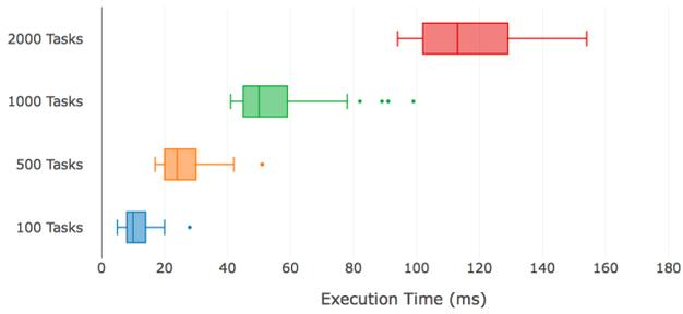
**Figure 7: Execution time of the QoD Controller, given a fixed amount of executing tasks and using two TMs.**
