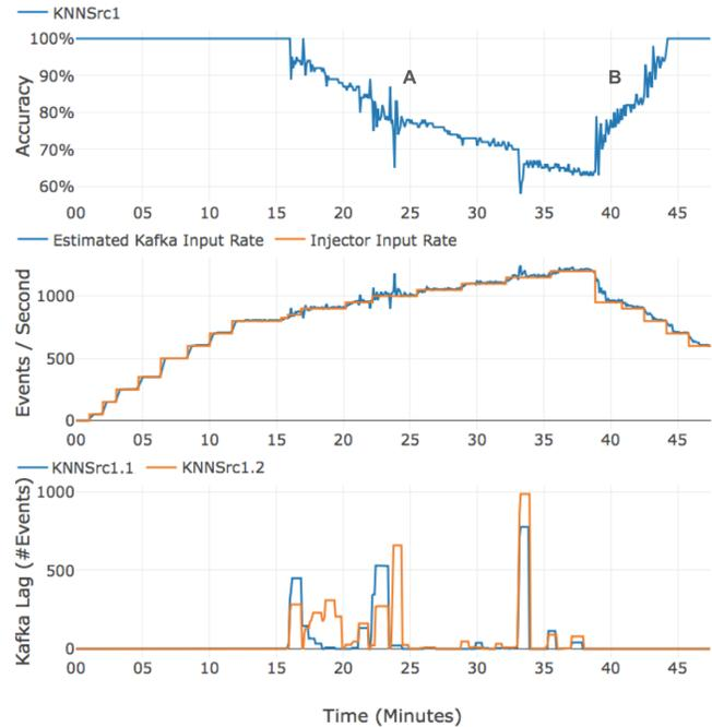
**Figure 5: Execution of the KNN application as the event injection rate changes. First chart shows its accuracy; second chart a comparison between the injection rate and estimated injection rate to the Kafka topic; and third chart, the Kafka topic partitions’ lag.**
