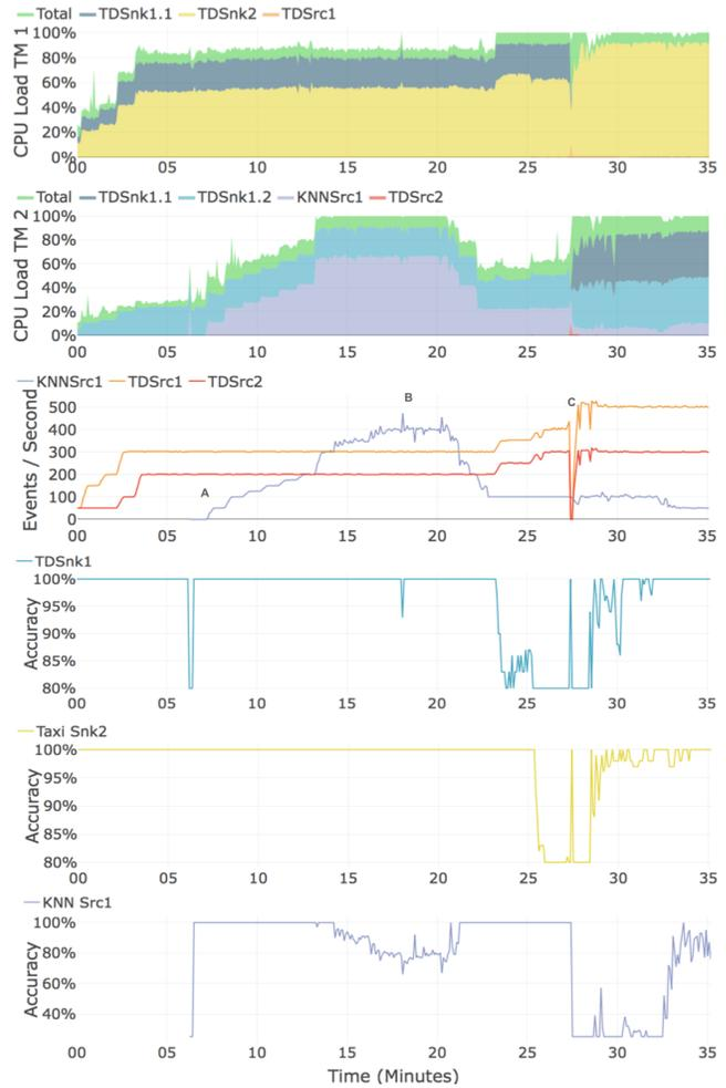
**Figure 4: TD and KNN applications execution, having tasks with different priorities. First two charts show the CPU load in both TMs. Third chart shows the applications' throughput for each input Kafka topic. The accuracy for each sink task is presented in the remaining charts.**
