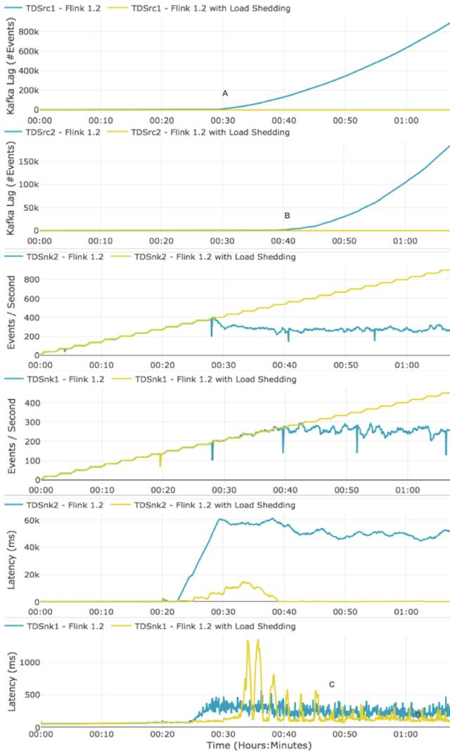
**Figure 8: Lag, consuming throughput and latency of the TD application as the injection rate increases, both when using Flink 1.2 and in our modified version of the same release.**
