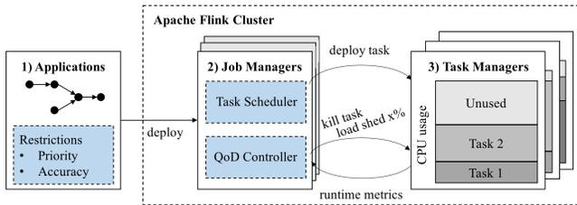
**Figure 1: Architecture and components of the proposed system in a Flink cluster.**
