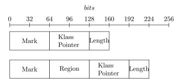
Figure 3.11: Layout of an array object header with an added word for BDA-region indexing
