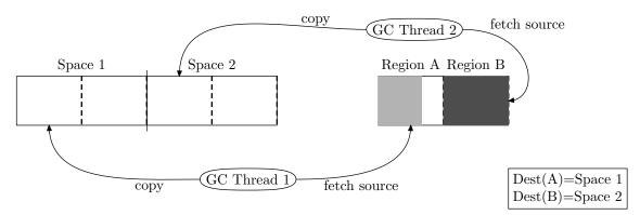
Figure 3.15: Compaction — fetching and filling of regions
