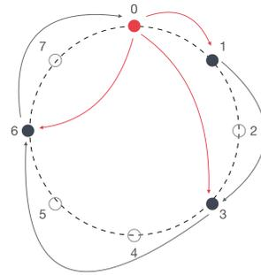
Fig. 11. Example of peer with ID = 0 fingers
