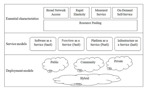
Figure 2.1: Cloud computing diagram.
