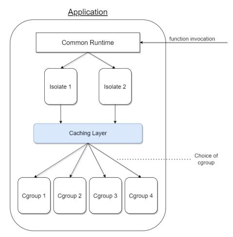
Figure 4.1: Architectural diagram with cache layer.
