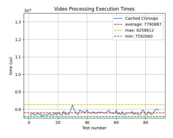
Figure 6.10: Video Processing Execution Times.
