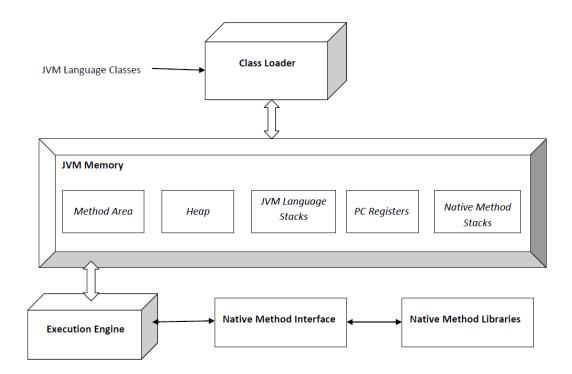
Figure 2.3: Java Virtual Machine architecture [1].
