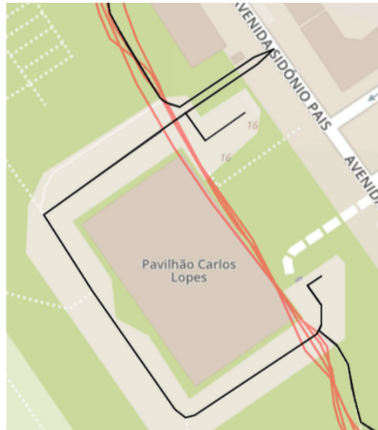
Figure 5.10: An example of an incorrect segment addition as a result of a lenient matching process. The user took a shortcut through the pavilion, but since there is not a corresponding path in the map network and the matcher candidate requirements were lowered to account for GPS errors, a round-about route was found instead of breaking the trajectory.
