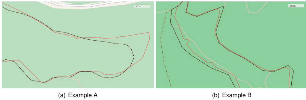
Figure 5.8: The map matching snapping effect. The orange line is the original trace, while the black line is the map-matched route. The traced line beneath the black line is the actual path.
