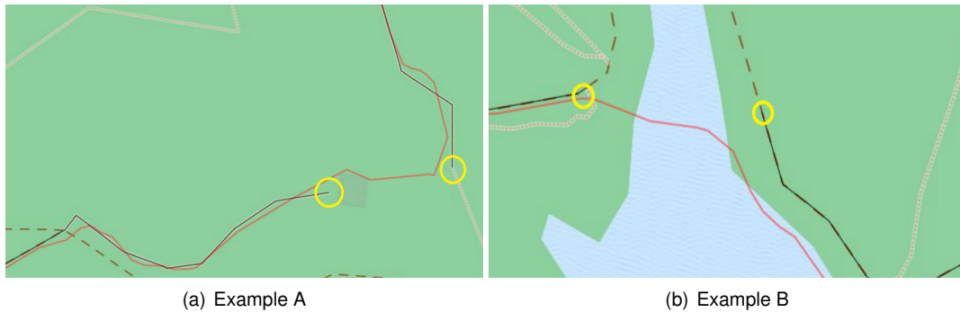
Figure 5.9: Map matching break on an incomplete path example. The breaks are shown as yellow circles.
