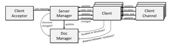
Figure 3. Server node components
