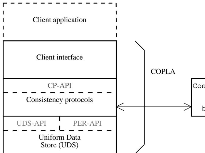
**Figure 1. COPLA architecture**
