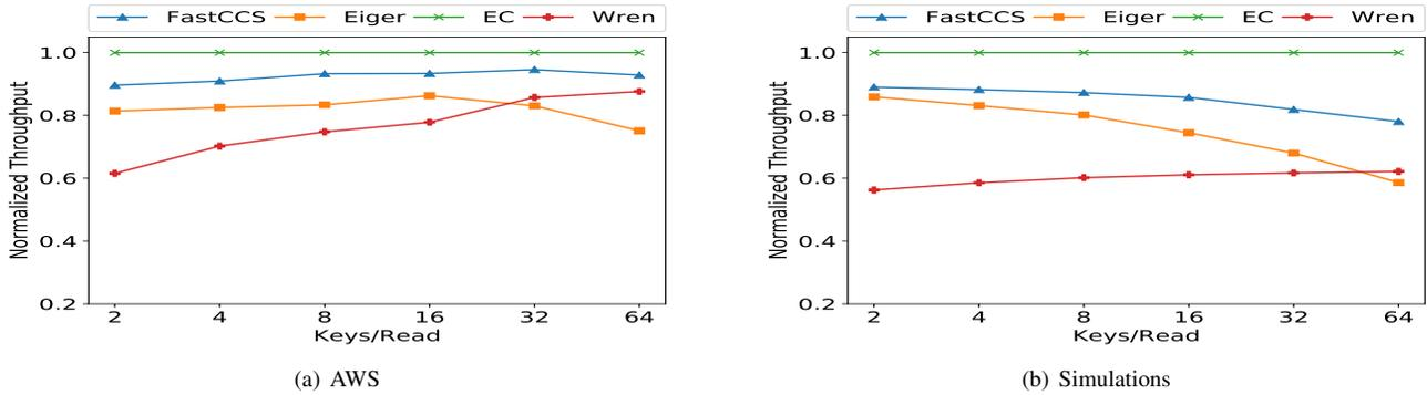
Fig. 2. Read throughput as a function of Tx length: AWS vs simulations.
