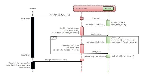
Figure 3.4: Execution of the challenge.  $set\_index_i$  is the index of a given file in the metadata vector, and  $block\_index_i$  is the index of a data block with size  $s_b$  inside the  $file_i$ .  $block_i$  is the read data block. sk is the secret key agreed between the auditor and the enclave.
