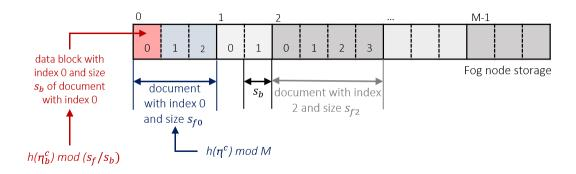
Figure 3.3: Fog node storage organization and hashes conversion to the first data block.
