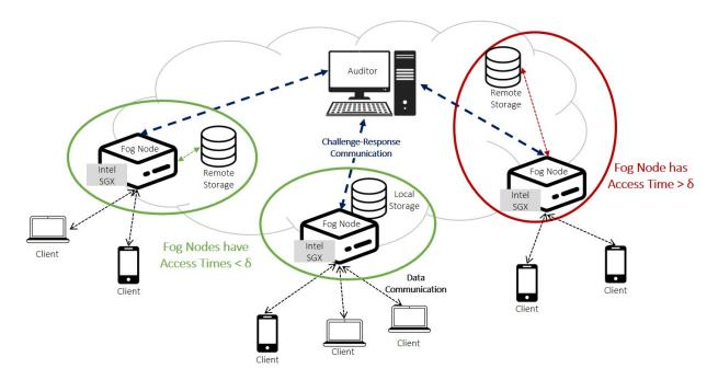
Figure 3.1: System architecture and communication channels.
