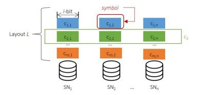
**Figure 2.2:** Storage layout L between n storage nodes.  $SN_i$  is a storage node;  $c_i$  is the verifiable version of a subfile  $f_i$ , and  $c_{i,j}$  is a l-bit block, also described as *symbol*.
