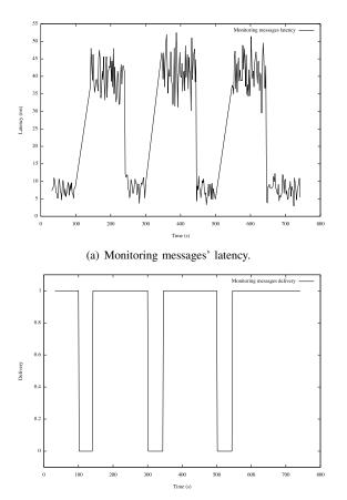
(b) Monitoring messages' delivery (Note: 1 is delivered, 0 is not delivered).
