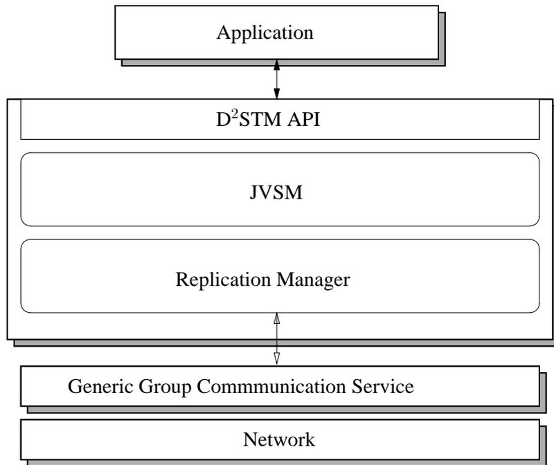
Figure 1: Components of a D<sup>2</sup>STM replica.
