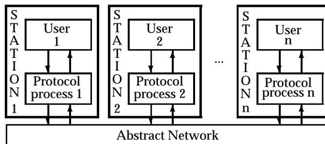
As already stated before, a set of scenarios is needed for the verification. Each of these scenarios describes a closed system containing the following processes (see the above figure for network configuration):
