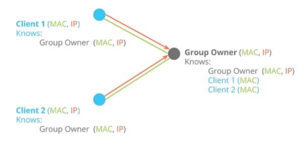
Unfortunately, the Wi-Fi Direct API does not give the group owner direct access to the IP addresses of the clients. The group owner only has access to its clients' MAC addresses. To get access the clients' IP addresses, initiate a socket connection from the client to the group owner.
