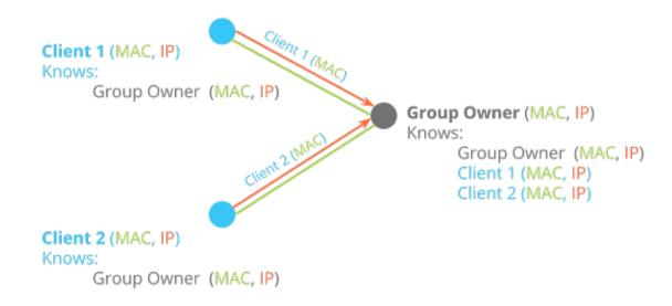
Once that socket connection is established, the client can send a string containing its MAC address to the group owner, so the group owner would be able to add the IP of the socket connection to the known MAC of the client, thereby creating a MAC, IP pair
