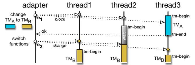
Figure 3: Switching TM algorithm safely in PolyTM.
