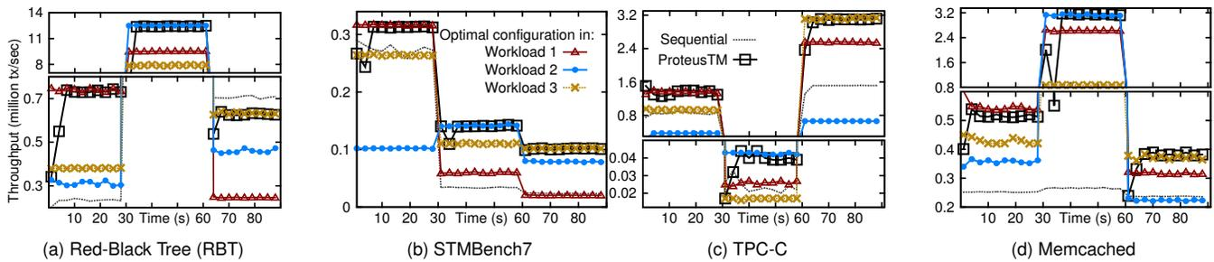
**Figure 7: Performance of four applications when their workload changes three times. It is shown the performance obtained with ProteusTM, and three additional fixed configurations, each one corresponding to an optimum in each workload.**
