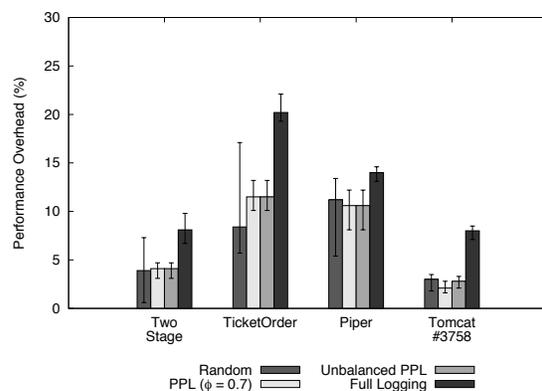
Figure 3: Performance overhead for the three partial logging schemes, as well as for a full logging strategy [8] (the error bars indicate the maximum and the minimum values observed).
