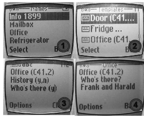
Figure 6: Phone book entries for preselected smart objects (1), a list of corresponding SMS templates (2), an edited SMS template with activated command (3), and the response message (4).
