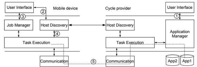
Figure 1: SPADE System Architecture
