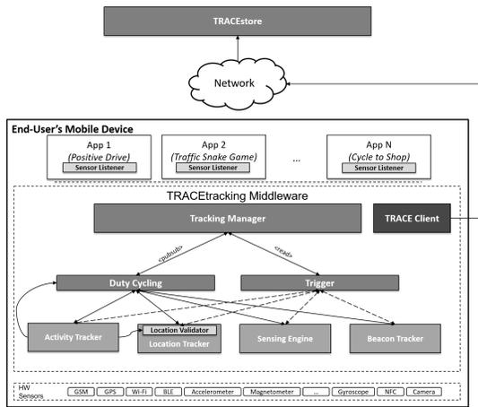
Figure 3: TRACE tracking module.
