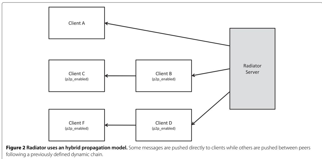
**Figure 2 Radiator uses an hybrid propagation model.** Some messages are pushed directly to clients while others are pushed between peers following a previously defined dynamic chain.
