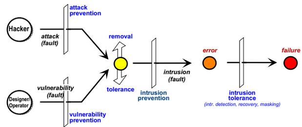
Figure 1. The Composite Failure Model of MAFTIA
