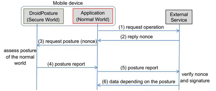
Fig. 2. DROIDPOSTURE providing a posture report to an external service.
