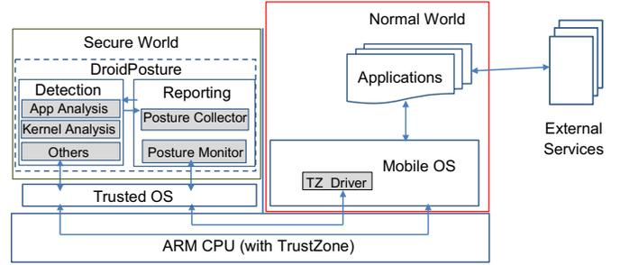
Fig. 1. Architecture of a mobile device running DROIDPOSTURE. The grey boxes are components of the DROIDPOSTURE service.
