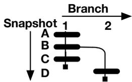
Figure 5. Tree model: 2 branches and 4 snapshots: branch 1 contains snapshots A,B,C; Branch 2 contains snapshots A,B,D.
