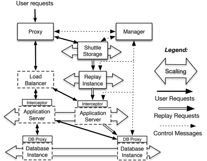
Figure 1. Shuttle architecture (PaaS components are dashed).
