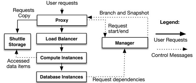
Figure 2. Interaction between components during normal execution.
