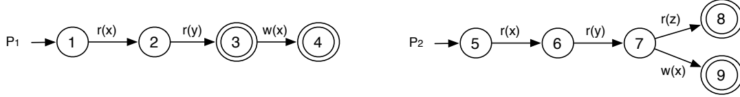
Figure 1: Sequential programs P_1 and P_2 with initial states 1 and 5 and final states \{3, 4\} and \{8, 9\} , respectively
