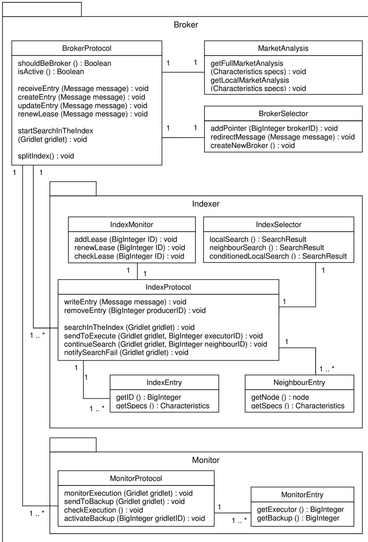
Figure 8 - Diagram of the broker module implementation
