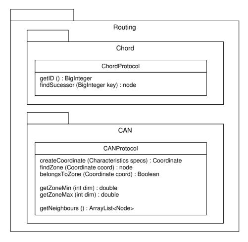
Figure 9 - Diagram of the routing module implementation
