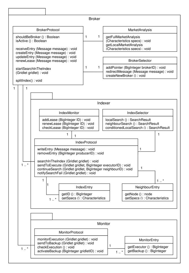
Figure 8 - Diagram of the broker module implementation
