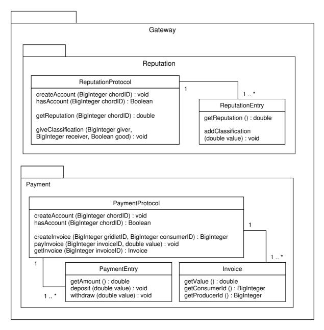
Figure 10 - Diagram of the gateway module implementation
