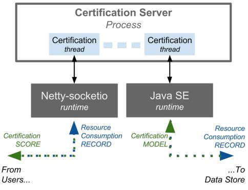
Figure 4.3: Certification Server Process and Threads.
