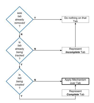
Figure 4.1: Tab State Consistency Flowchart.
