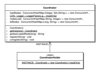
Figure 3.9: Coordinator package class diagram
