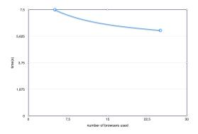
${f Fig.\,17.}$  Time elapsed on a ray-tracing job divided in 25 computing units
