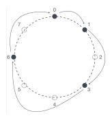
${\bf Fig.~10.~Minimum~number~of~connections~for~messages~to~be~routed}$  properly
