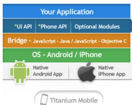
Figure 2.3: Titanium Mobile Architecture Overview
