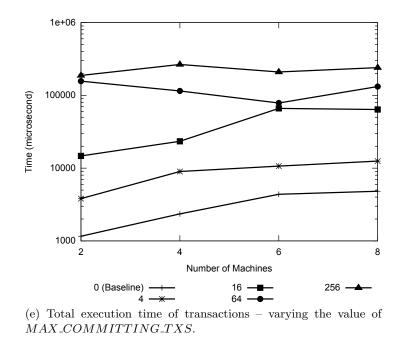
Figure 4.2: Bank Benchmark – Configuration B.
