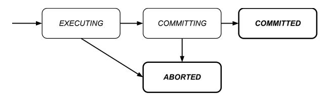
Figure 2.1: The life of a transaction.
