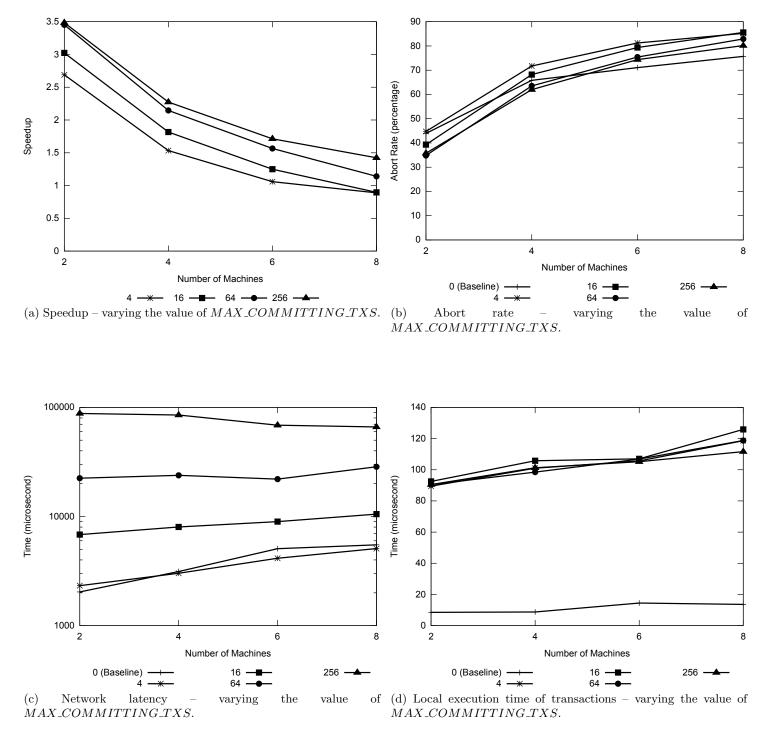
Figure 4.2: Bank Benchmark – Configuration B.
