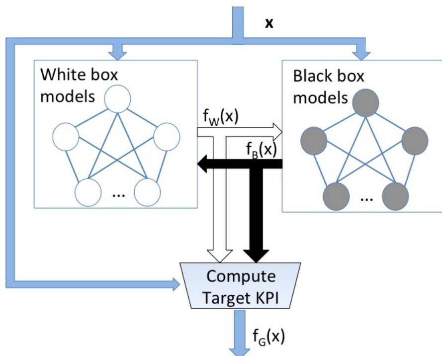
Figure 4.1: Design of the *Divide et impera* performance modeling technique.
