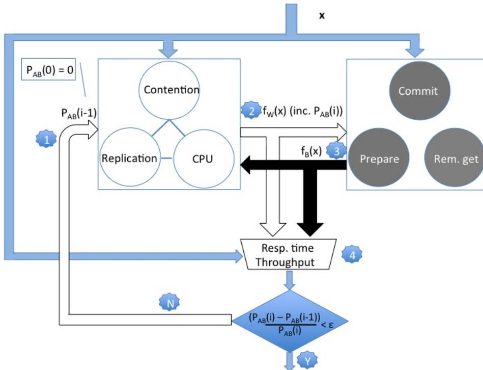
Figure 4.2: *Divide et impera* applied to DTPs performance modeling.
