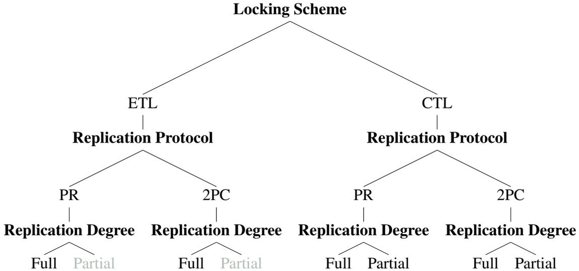
Figure 1.2: DTPs design space dimensions considered in this dissertation: replication degree, replication protocol and concurrency control scheme. Leaves of the tree marked in black correspond to design choices for which this dissertation presents a performance model; lighter gray, instead, denotes combinations that are not addressed. The motivations behind the exclusion of specific combinations are discussed in Chapter 4.
