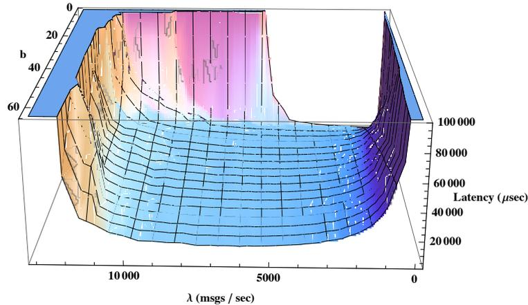
Figure 5.2: Messages delivery time of the STOB service as a function of  $\lambda$  and  $b$
